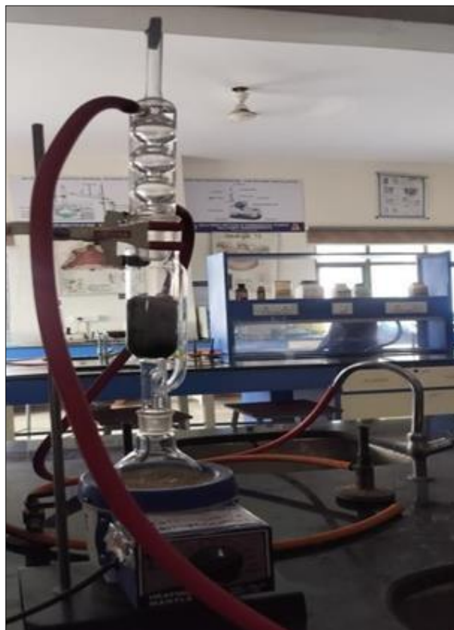
Fig 6: Soxhlet extraction of Pothos scandens leaves powder
