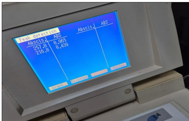
Figure 1: Wavelength of Maximum Absorption ( \lambda_{\max} ): The UV-spectrophotometric scanning revealed that the maximum absorption ( \lambda_{\max} ) for paracetamol in 0.1N NaOH solution occurred in the range of 256-258 nm. The average \lambda_{\max} was determined to be approximately 257 nm, which is consistent with literature values for paracetamol in alkaline medium [1, 10].
